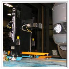
unique feature on the wheel and determines it's orientation. Virtual real time measurement updates are then performed which reduces machine cycle time by 3 or 4 seconds for every adjustment made. If several adjustments are made the cycle time decreases even more
