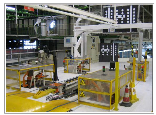
The driver can see on the screen a live view of the rear part of the vehicle. The system indicates in the display the approximation to an obstacle and warns acoustically by small distances between the car and the obstacle. The Fori Unit provides a reference sample (installed behind the vehicle on the hall floor). The rear view camera takes a picture of the sample, and the calibration is independently calculated in the car controller.
